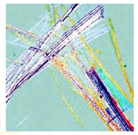
The scientific and commercial properties of asbestos were soon recognised. Asbestos has the ability to resist corrosion, has excellent thermal insulation properties and can sustain high temperatures without deterioration. Although substitutes have been developed to replace individual asbestos applications, nothing has ever been found or created which has all of the properties of this mineral.
